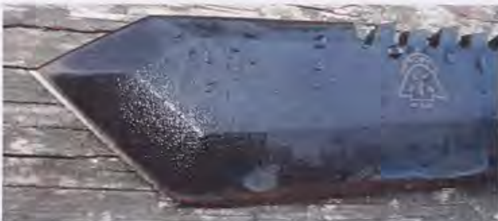
The thickness of the blade (3/16 inch), which travels nearly to the tip, the sharpness of the point, and the two sharp sides of the blade lend themselves to fantastic penetration.
